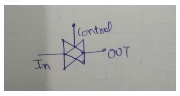
It is bidirectional switch, turned on/off through a contro, line when control signal is 1, it is in on state
