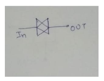
tran gate is bidirectional gate of two ports, when instaniated it connect the two ports directly
