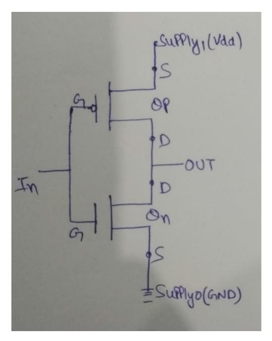
Cmos inverter formed by connecting an n-mos and a p-mos switch in series across the supply.the output terminal are joined together to form the common output
