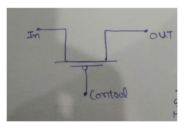
When control is at high state, the switch if off.
