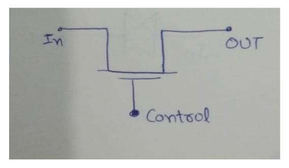
When control input is at (1) high state, the switch is on. It connects the input lead to the output side and offer zero impedence.
