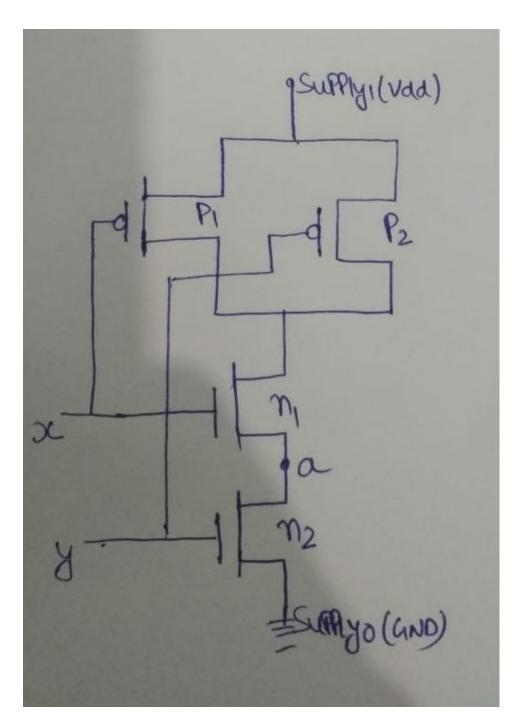
Cmos nand gate consist of two pmos and two nmos gates
